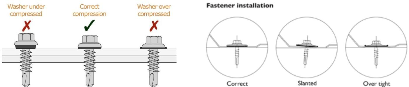
*TIP: Make sure fixings are not over tightened as this can burn off the soft neoprene pad under the washer*
